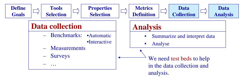
**Test bed**. An environment containing the hardware, instrumentation, simulators, software tools, and other support elements needed to conduct a test.
