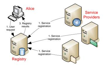
Fig. 1. Centralized Registry and Matchmaker
